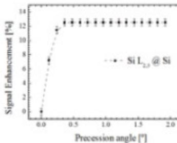
Signal enhancement as a function of precession angle for the Si L<sub>2,3</sub> edge in a Si crystal in <110> zone axis conditions.
