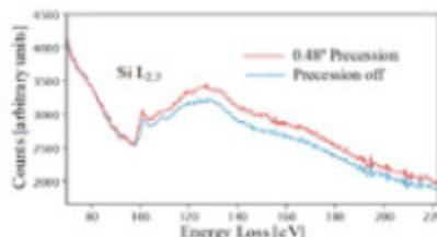
0.48° precessed and precession-less EEL spectra showing the Si L<sub>2,3</sub> edge in a Si crystal in <110> zone axis conditions.
